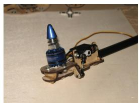
I mounted the motor plates and yaw assembly to the booms using a dab of household Goop. Works well, and will allow you to make repairs if necessary. I used relatively short arms (about 7 3/4" for front arms, and about 6 1/2" for rear arm). This gave a nice size.
