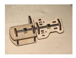
One mod I did to the top plate was to install 4-40 blind nuts to match the hole pattern of the stabilization board. I also soaked the ply around the tab/slots with thin CA and let everything dry thoroughly.
