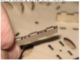
As you can see in the picture, I used a small "persuader" to tap the pieces together. This made for a very nice tight and square fit.
